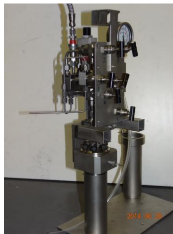
Figure 2: Manufactured autoclave undertaking 50 bar pressure test.
