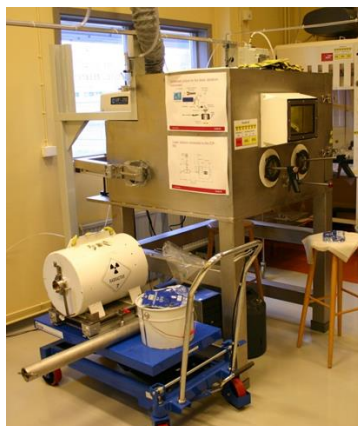
Figure 1: The laser ablation hot cell and the sample transfer cask.
