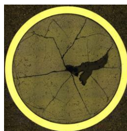
Figure 3: Optical micrograph of the microstructure of the spent fuel sample (the large dark part is due to a missing part of the fuel lost during the sample preparation).
