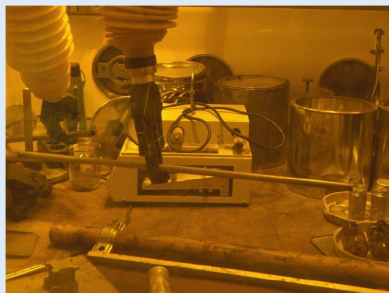
Fuel rod segment at the shielded box-line of KIT
